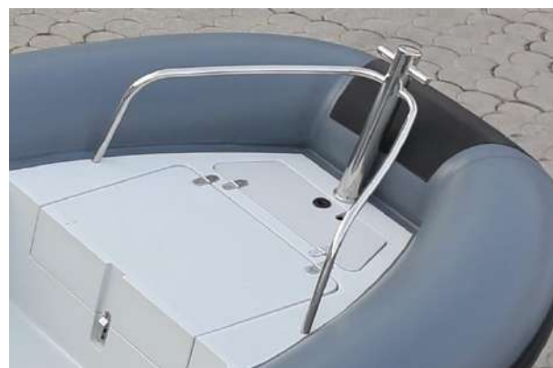
BOW MOORING CLEAT WITH HANDRAIL
