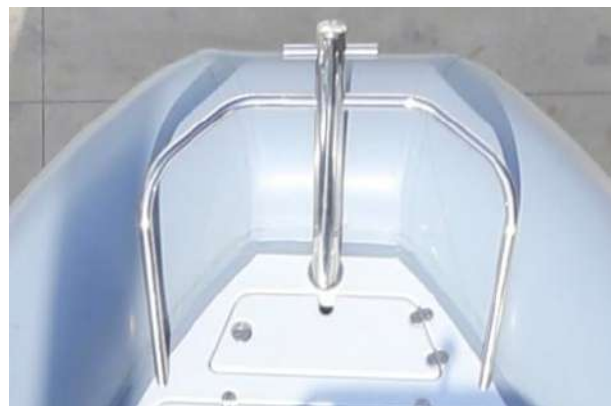
BOW MOORING CLEAT WITH HANDRAIL
