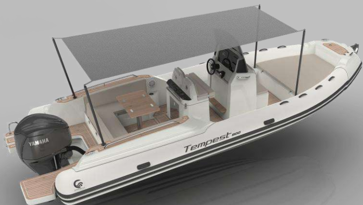
BIMINI (4 carbon pylons)
